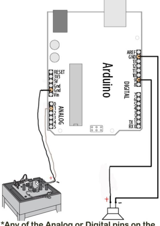
\*Any of the Analog or Digital pins on the Arduino board could be used
