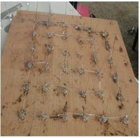
You solder every short LED leg so that it connects to the next. This step was repeated five more times in order for me to have the complete six layers. Along the way I also had to be careful of the longer LED leg that was left untouched so that it wouldn't interfere with the electricity being sent to the short leg. After I finished making the layers, I now how to stack them vertically. The
